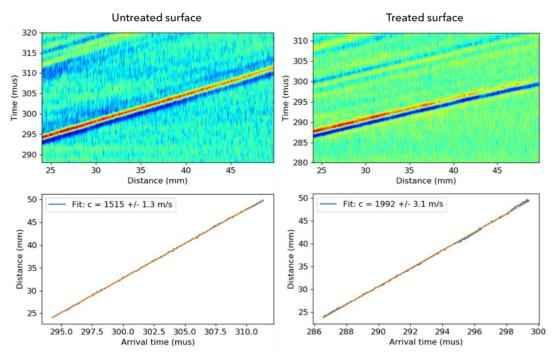
**Figure 6:** Guided wave propagation velocity along untreated and treated sandstone surfaces. The upper panels show B-scans from the untreated and treated surfaces, respectively. The main component of the guided wave is a transient with ~2  $\mu$ s duration, identified as a Rayleigh wave. Lower panels: Tracking the minimum of the transient and linear regression yields propagation velocities in good correspondence with previously published measurements on the sample.
