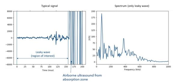
**Figure 5:** Typical signal and spectrum from measurements on the sandstone samples. Left panel: Similar to the measurements on metal plates, a guided wave precedes air-coupled acoustics from the absorption zone. Right panel: The recorded guided wave signal contains frequencies from a few kHz up to 800 kHz.
