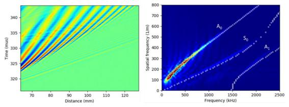
**Figure 4:** Acoustic dispersion in an aluminium plate. Left panel: B-scan compiled from signals recorded at different distances between excitation laser spot and detector. Right panel: 2d Fourier transform of the B-scan, leading to an array with amplitudes over spatial frequency and temporal frequency. Maxima correspond well to the different Lamb dispersion curve branches calculated numerically (grey dots).
