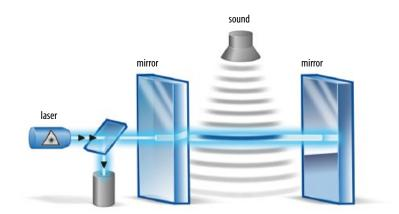
Fig. 2 Principle of operation of the optical microphone. The ultrasonic signal is detected optically by the change of the refractive index within a Fabry-Pérot etalon.
