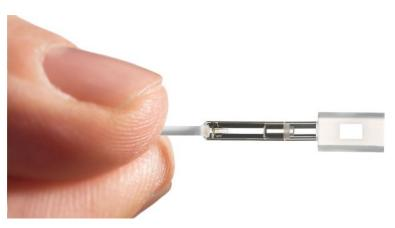
Fig. 1 Sensor head connected to an optical fiber: centerpiece of the optical microphone is the miniature Fabry-Pérot etalon shown on the right side of the picture. Sound enters the etalon through the air gap between the mirror surfaces. Small size and robust dimensioning of the glass elements prevent the influence of mechanical vibrations to be below the sensor self-noise throughout the full measurement range.
